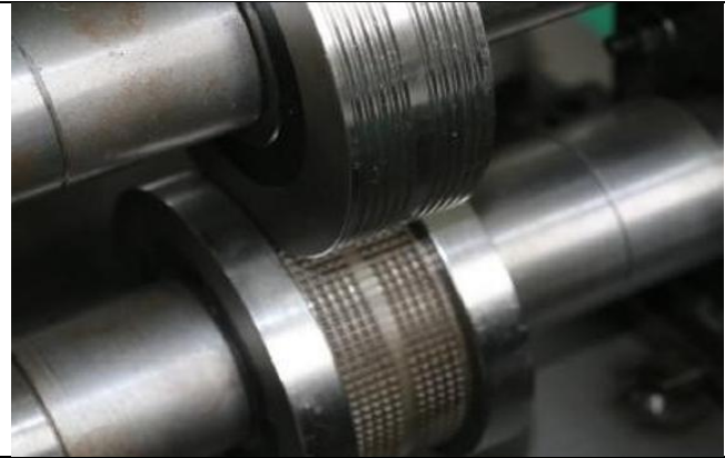
The roller to make the knurling on the product
