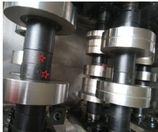
The roller to make the knurling on the product
