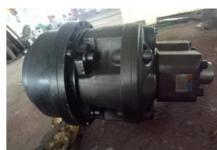
The upper roll is a driving roll of four roll rolling machine (as shown below). The independent hydraulic motor on the upper roll and the high-power box are directly coupled (straight), not through the intermediate gear transmission, which is the most energy-saving drive method. The hydraulic motor is equipped with an immediate brake to allow the roll to stop accurately in the pre-bending state.
