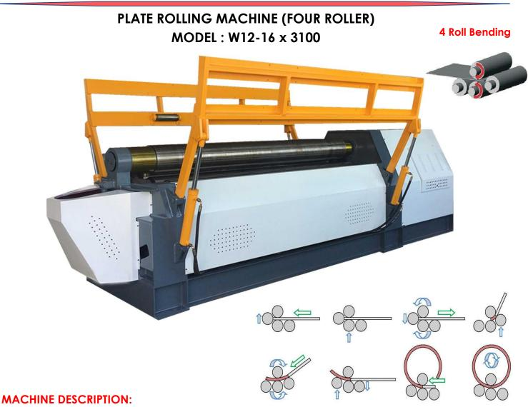
The equipment has the pre-bending function of the plate end and the CNC rolling function. It can feed the metal plate at a time, and can complete the pre-bending and the roll forming of the work piece without turning the head.
