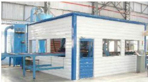
Housing and Dust Collector
